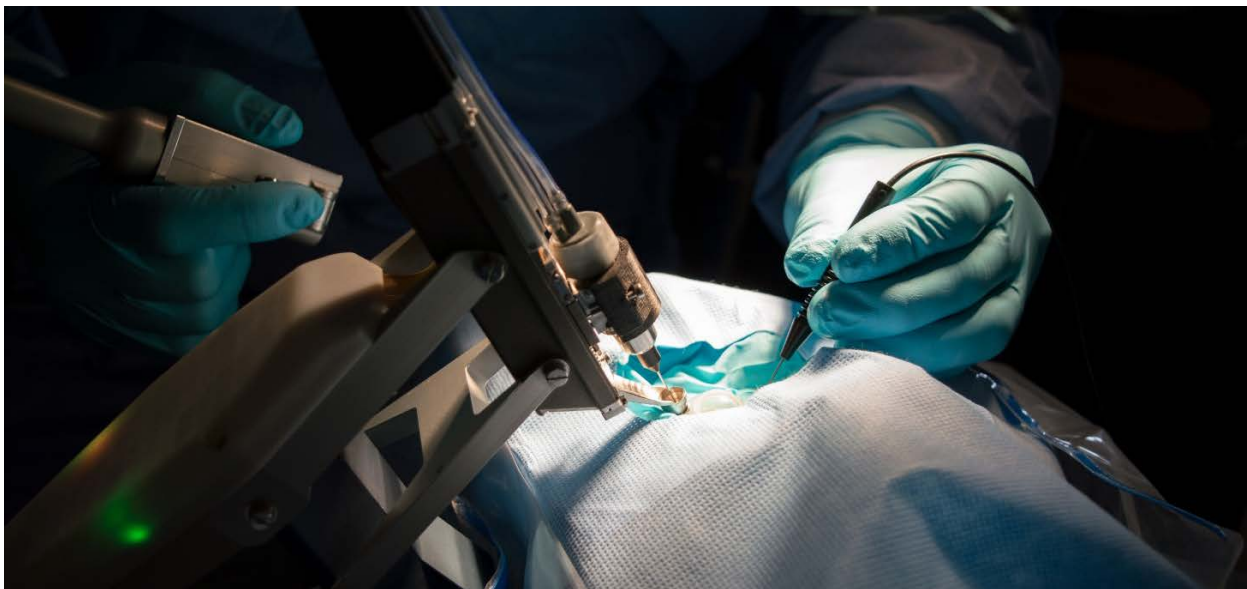
The robotic manipulator of the PRECEYES Surgical System holds and positions a surgical instrument inside the eye, following positioning commands that the surgeon provides with a controller.
