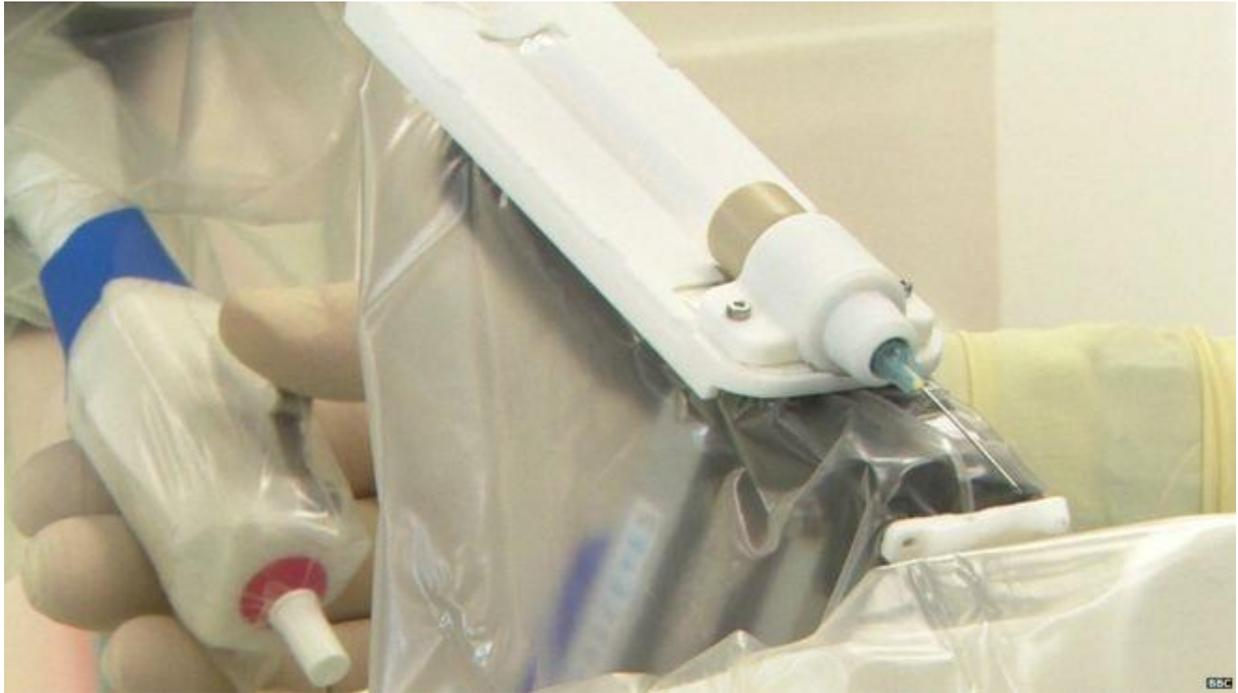
The PRECEYES Surgical System manipulates the instrument that enters the eye and is controlled using the motion controller on the left - Copyright and courtesy of BBC.
